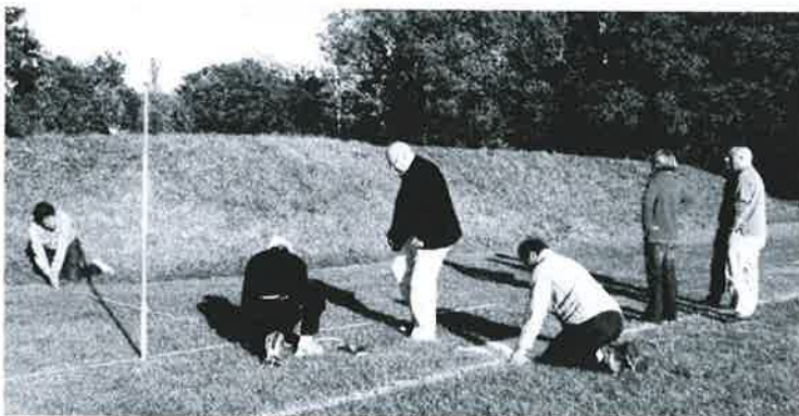
Locating the precise position and shape of the Oakley mound, using baseline and offset
