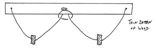
This is how it works. Two beads are threaded on twine, which is secured at each end of a batten by a knot behind a small hole. The twine passes through a larger hole in the centre of the batten, making a loop and noose. The beads are too big for the hole (the twine may be longer than shown).
