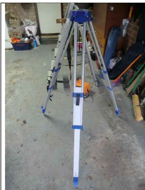
Erected tripod – note clamps approx. half way down each leg.
